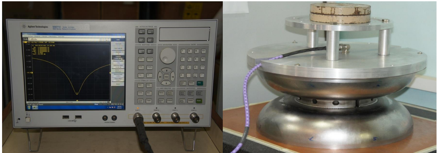
RF qualification of a 650 MHz 0.92 Beta dumbbell structure. A copper clad RF laminate is used at the bottom and at the top equator to ensure good electrical contact. The VNA signal shows the S11 for the cavity structure.
